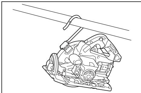
Attach the hook with the screws as illustrated.
