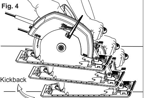
1. Maintain a firm grip and correct body position. Position arms and body to control the upward and backward reaction force of kickback (Fig. 4).
