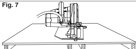
6. Always allow blade to come to a full stop before removing the saw from the workpiece. Never remove the saw from a cut while the blade is moving. If restarting or correcting direction in mid-cut, allow blade to coast to a stop, back saw up a few inches and center it in the kerf before restarting.
