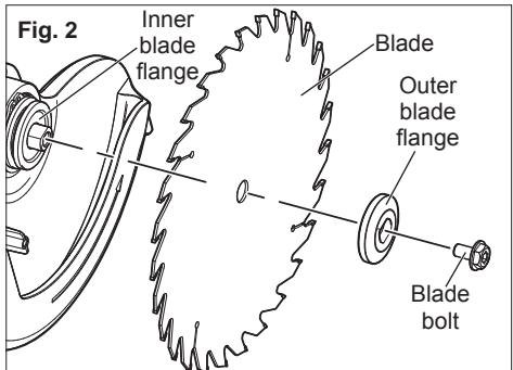
3. Push lower guard lever up to raise lower guard. Place blade on spindle with teeth pointing the same direction as the arrow on lower guard. Release lower guard lever.
