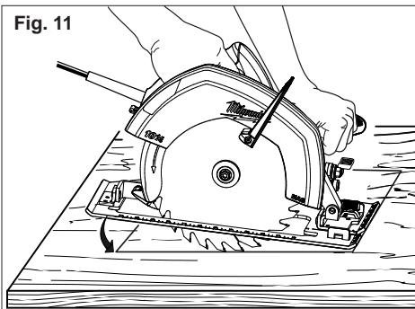
3. When shoe rests flat against workpiece (Fig. 12), move saw to far corner. Release trigger and allow blade to come to a complete stop before removing it from workpiece. Repeat the above steps for each side of the opening. Use a Sawzall®, jig saw, or small hand saw to finish corners if they are not completely cut through.
